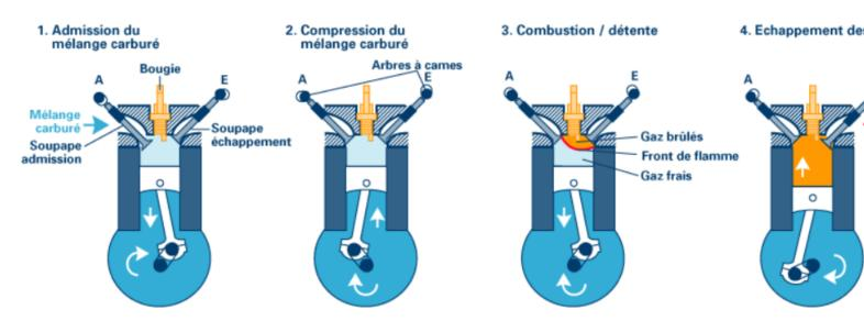
For a compression ignition and direct injection diesel engine, the 4 strokes operate in the same way, with two differences:
