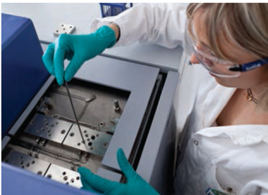
Loading of reactors on HTE equipment.
