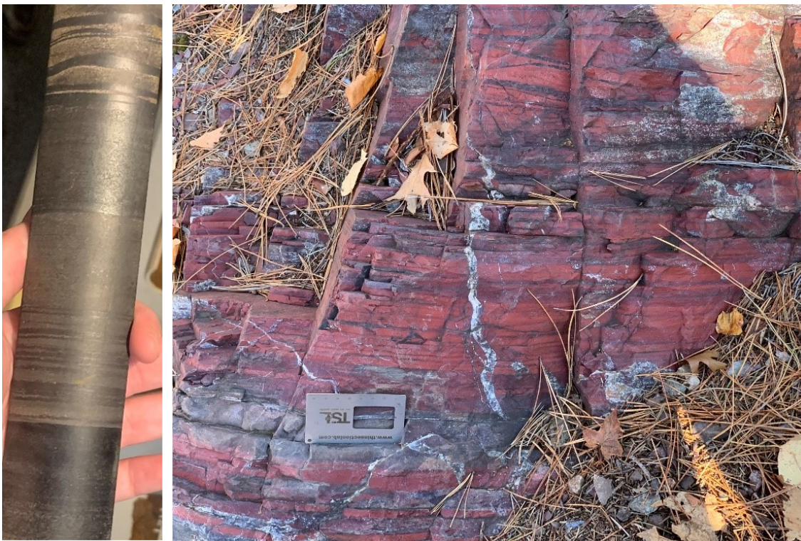
Figure 1a: Reduced BIF core taken from a depth of several meters (Hamersley Range, Australia); 1b: Oxidized surface BIF in northern Minnesota (credits: Olivier Sissmann)
