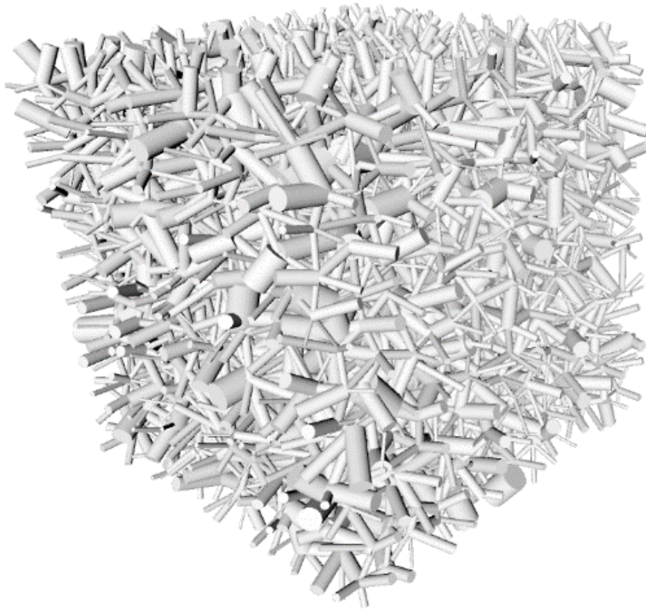
Figure: Representative Elementary Volume of the digital twin of a real alumina.
