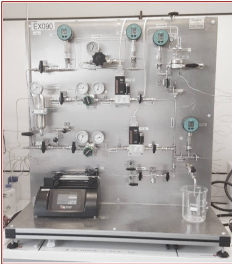
In situ analysis unit for the Quick-XAS monitoring of catalyst activation in industrial conditions.
