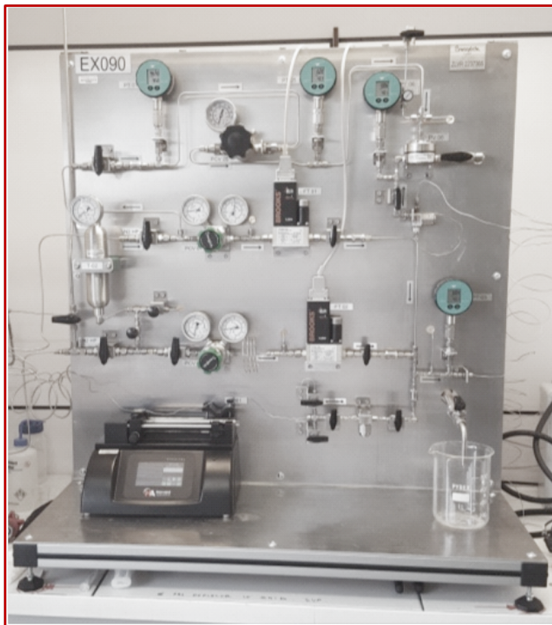
In situ analysis unit for the Quick-XAS monitoring of catalyst activation in industrial conditions.
